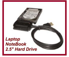
The 2.5" IDE Drive has one connector on the rear. This 44 pin connector is IDE DATA and IDE Power combined. This connector has a blocked socket and must be installed in the correct orientation. Match the blocked socket with the missing pin on the drive mechanism.
