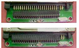
Position the disk drive onto the circuit board then align the left side pins with the 44-pin IDE connector.
